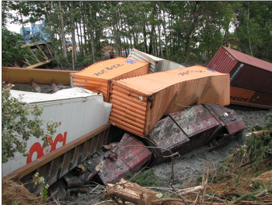
Photo 2. Cars piled up on top of locomotives
