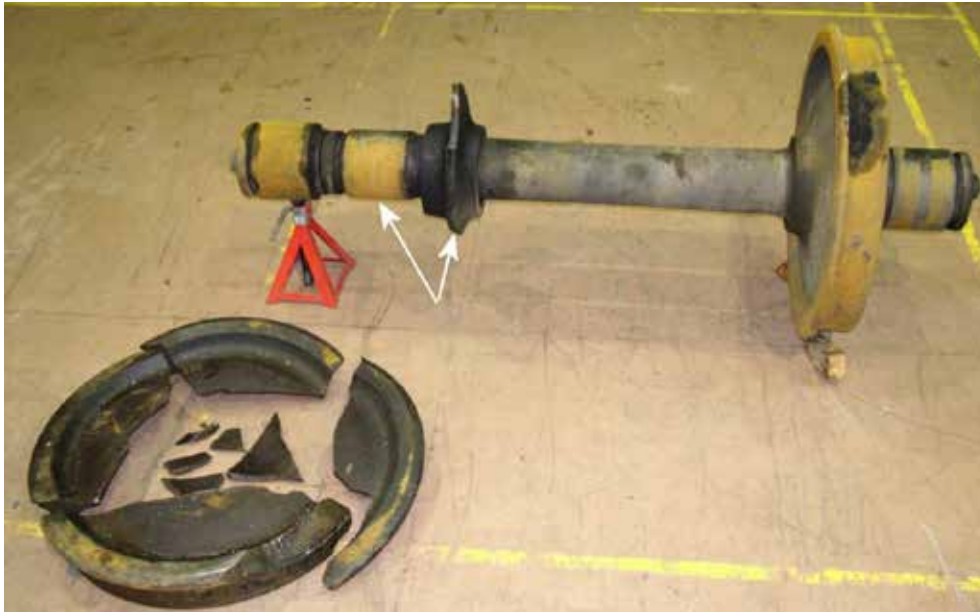
Photo 1. Broken L2 wheel and mate wheel
