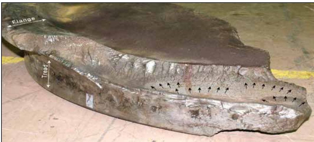
Photo 3. Arrows show the beach marks indicative of a progressive fracture.
