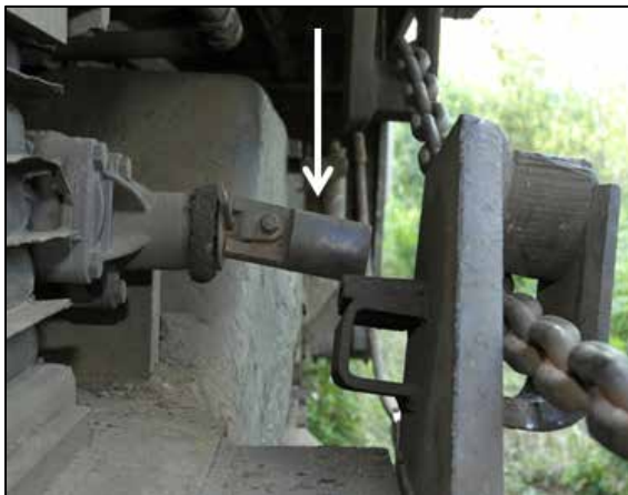
Photo 10. QRB valve used to exhaust brake cylinder air during hand brake application
