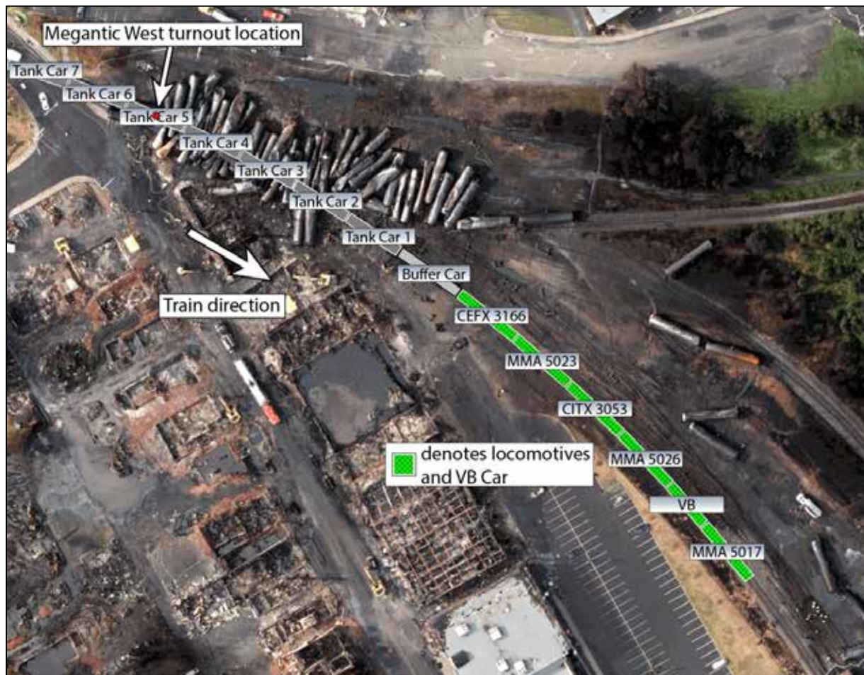
Photo 29. Location of the train when the brake pipe pressure dropped to 0 psi (sources: AeroPhoto and locomotive event recorder data)
