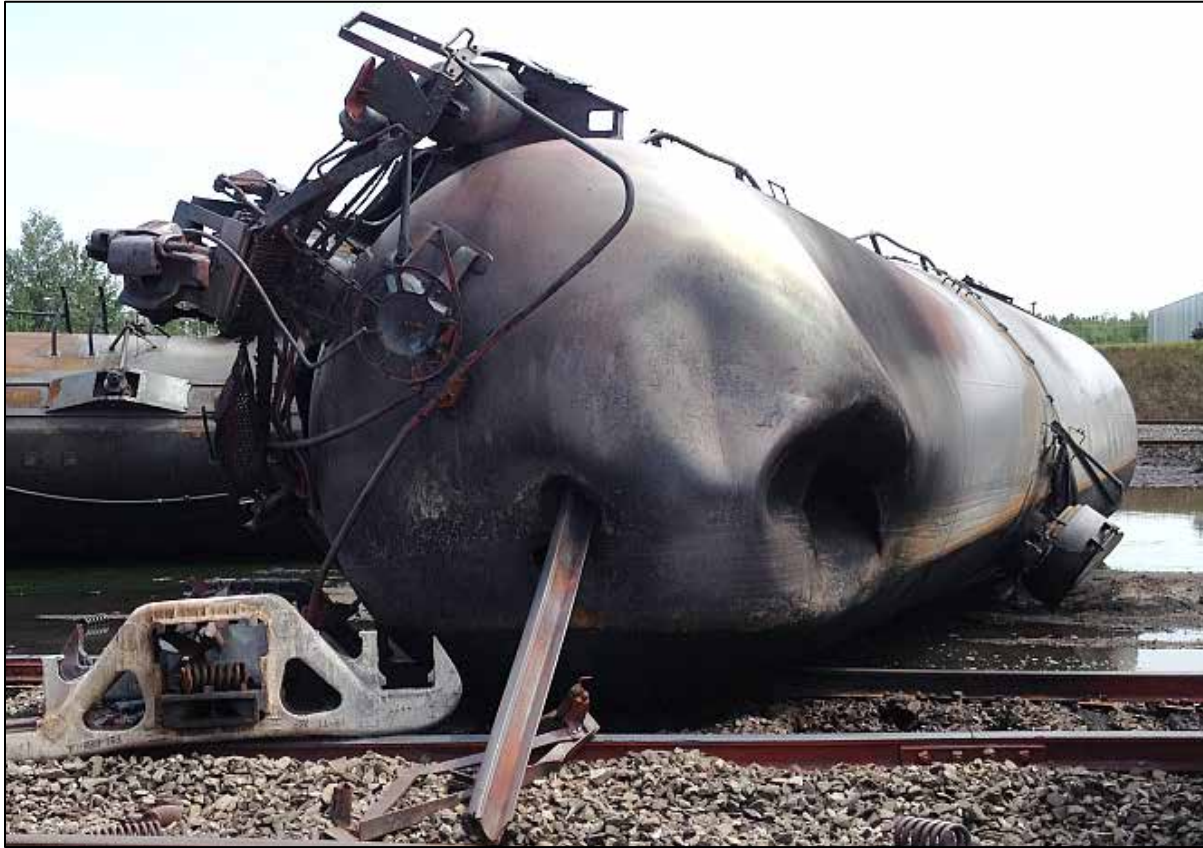
Photo 20. Head puncture due to rail impact
