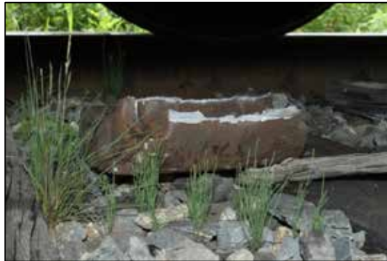
Photo 8. Broken locomotive knuckle segment found under the second locomotive
