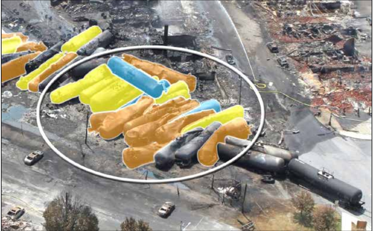
Photo 30. Concentration of large (orange) and medium (yellow) breaches toward the end of the derailment
