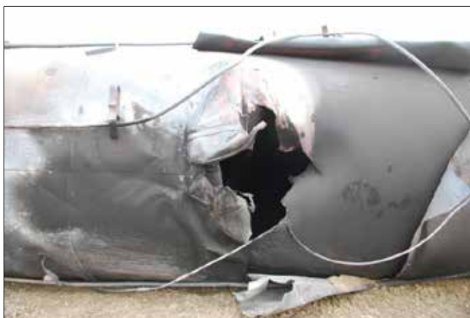
Photo 1. Puncture in the underside of UTLX 955375
