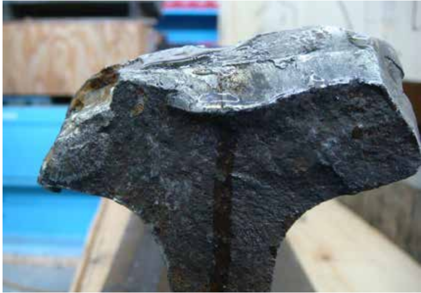
Photo 9. Wheel impact damage on rail specimen TSB-3 (Source: Exova)
