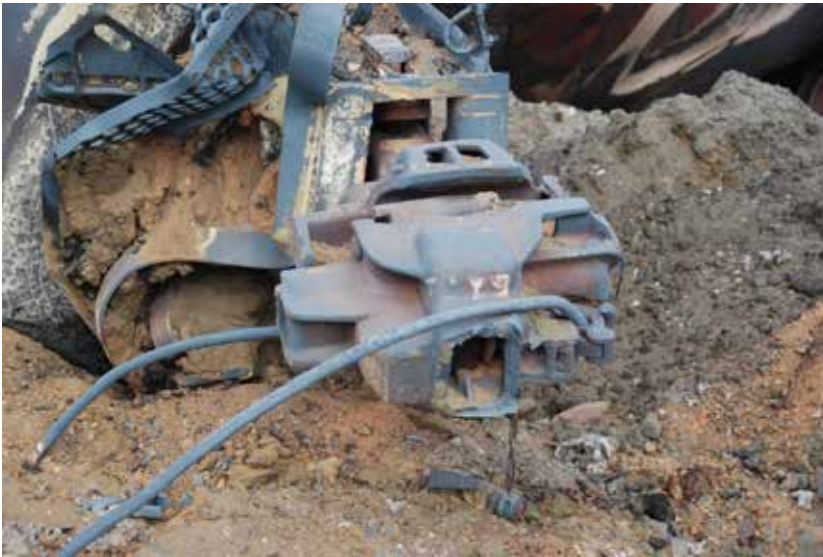
Photo 4. Coupler shank failure with the double shelf couplers still engaged
