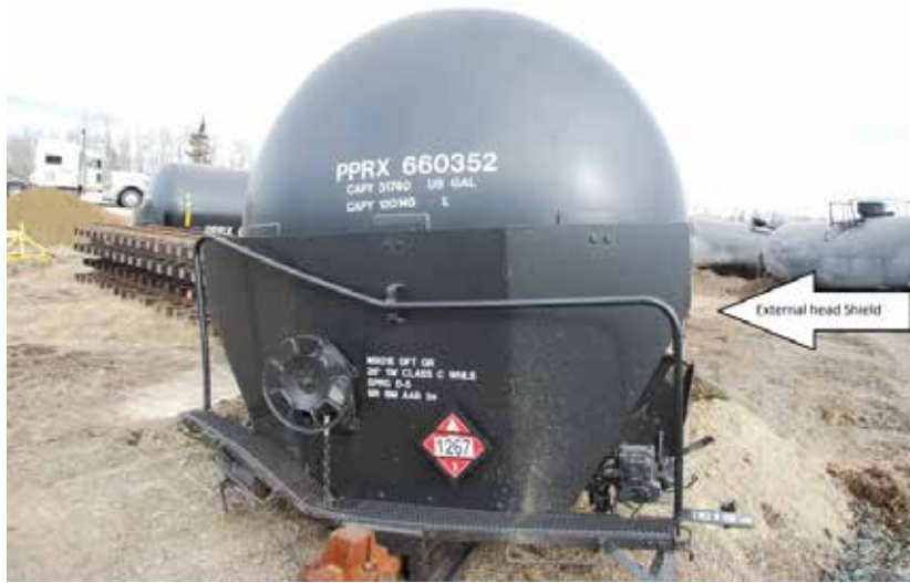
Photo 3. Head shield protection incorporated into tank head
