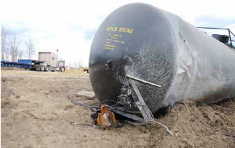
Photo 3. Head shield protection incorporated into tank head
