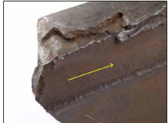
Figure 5. Shelling on the running surface at one end of the rail section
