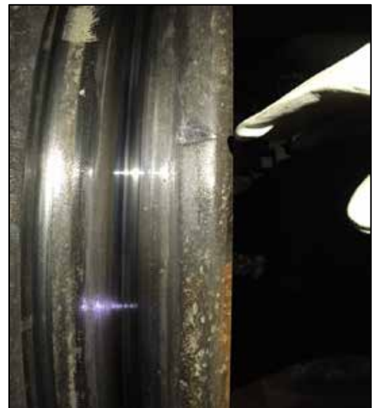
Figure 3. Impact marks on the north-side wheel of CNPX 3795, the 105th car (Source: Canadian Pacific Railway)
