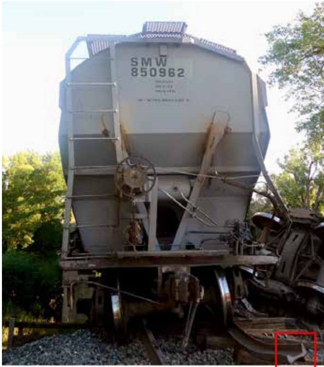
Figure 3. Looking south at the bridge's north approach with the failed thermite weld highlighted
