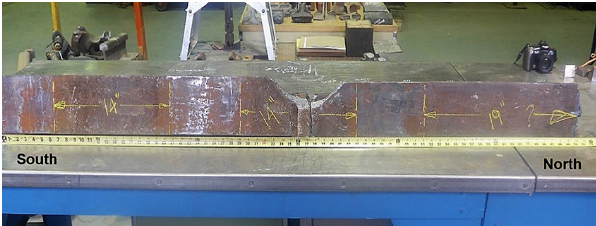
Figure 8. Tie spacing, as observed on the base of the rail
