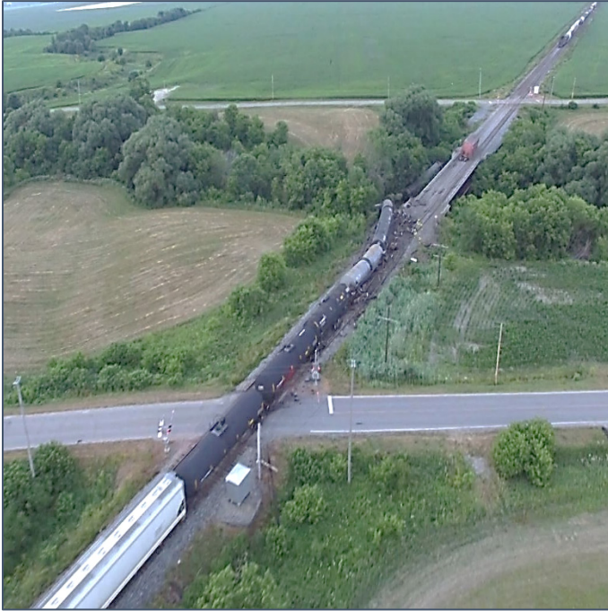
Figure 4. The 12 cars (24 platforms) that derailed about 700 feet west of Élie-Auclair Road crossing, looking east (Source: Third party, with permission)
