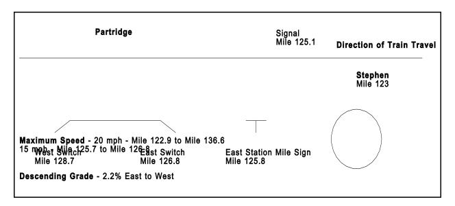
At Mile 125.1, the crew observed an "Advance Clear to Stop" signal indication which means "Proceed, next signal is displaying Clear to Stop, be prepared to stop at second signal." The next signal was at the east switch at Partridge, at Mile 126.8, and the second next signal was at the west switch at Partridge, at Mile 128.7.
